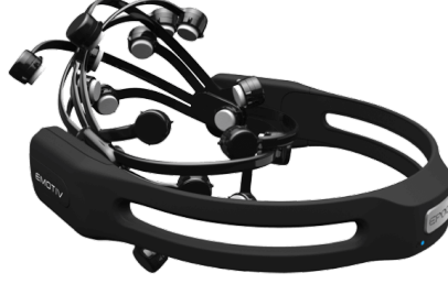
Figure 4.3: EPOC+ EEG used for signal acquisition [5].
